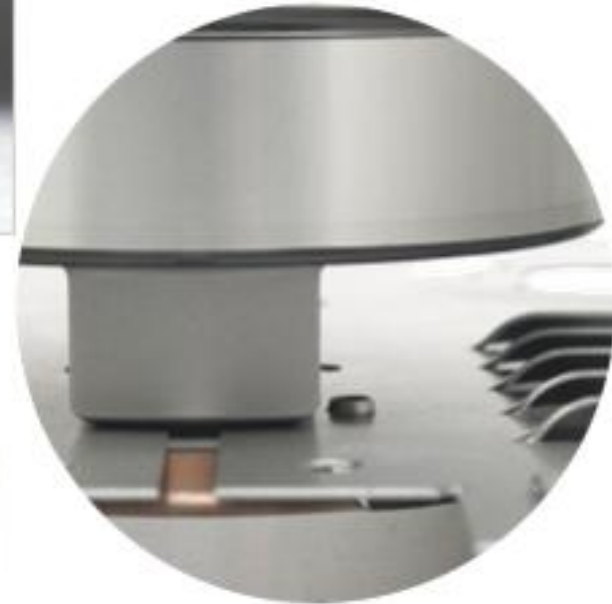
Fully Guided 'Clamp Clearing' Slitting Solution for punching close to clamps and forms
