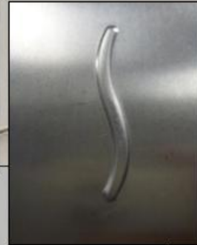
Emboss-up and emboss-down in one single hit
