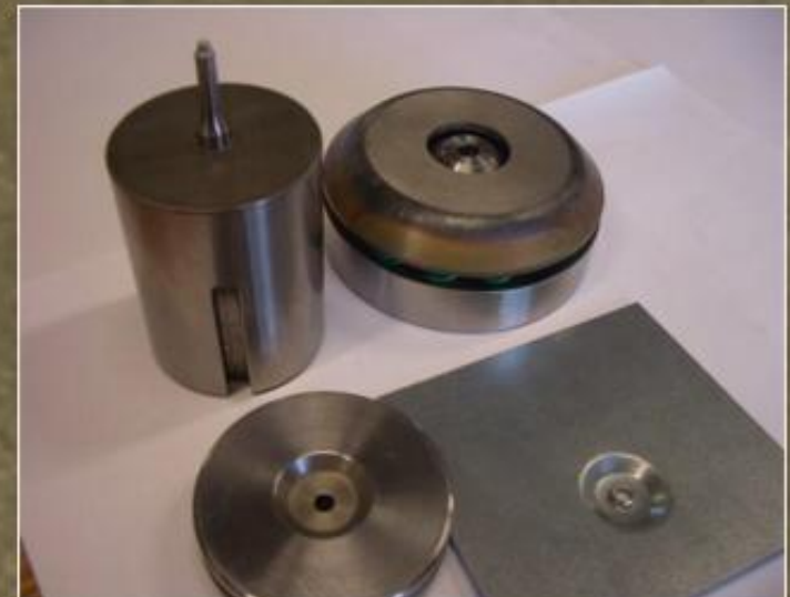
Pre-pierce, extrusion and emboss in one single hit
