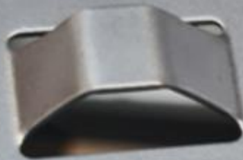
6.4mm high bridge in 0.7mm mild steel, with pre-punched sides (obround)
